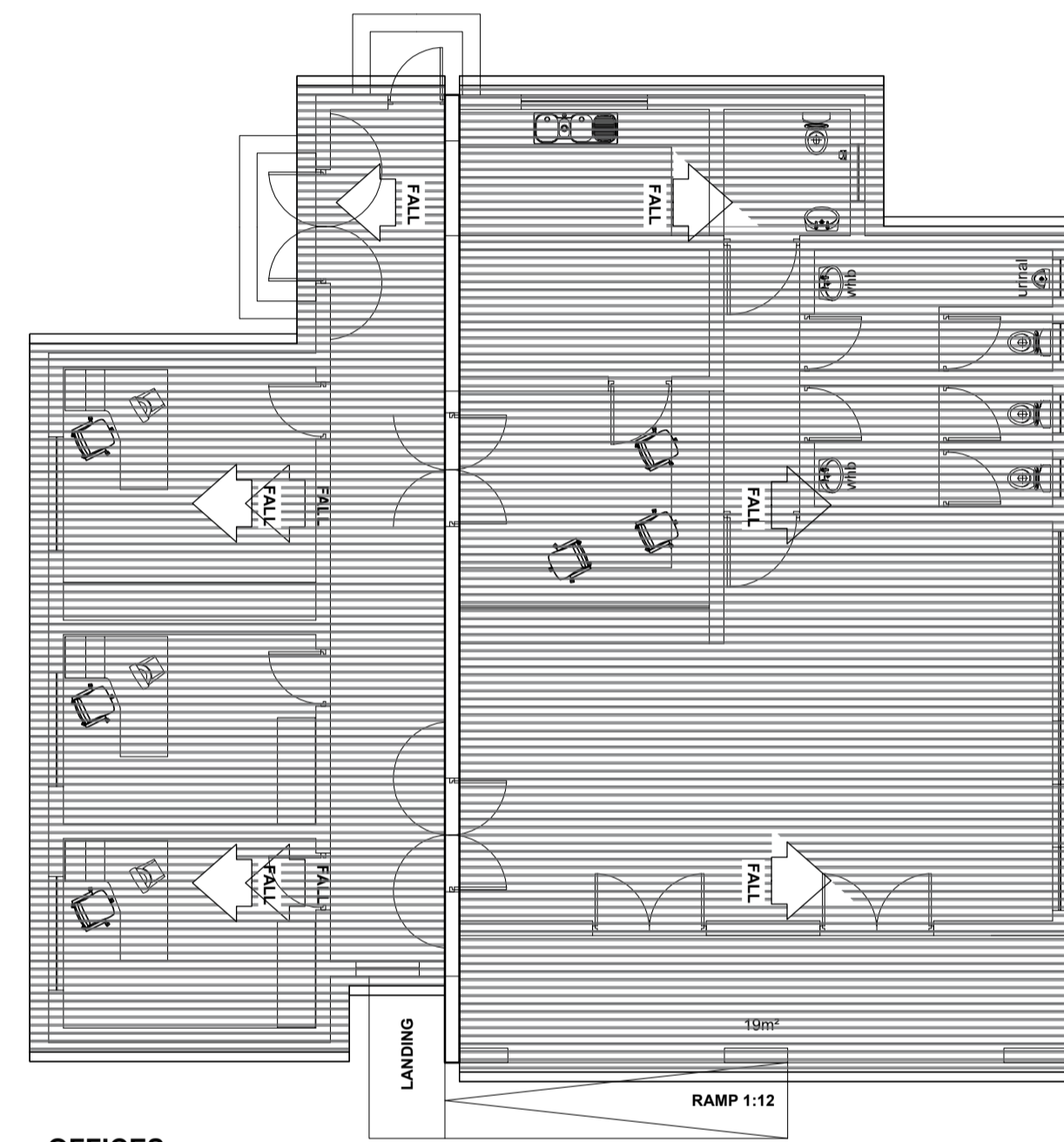
OFFICES ROOF PLAN scale 1:100
